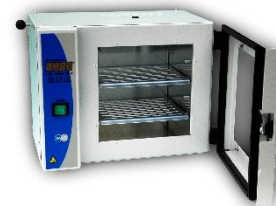
Incubator with adjustable temperature settings. Petri dishes can be placed in it.
